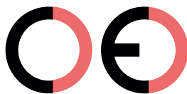
False CE Mark (too far)
